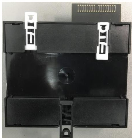
Figure 19: Top DIN Clip is shown removed from the base to mount the DIN clip separately.
