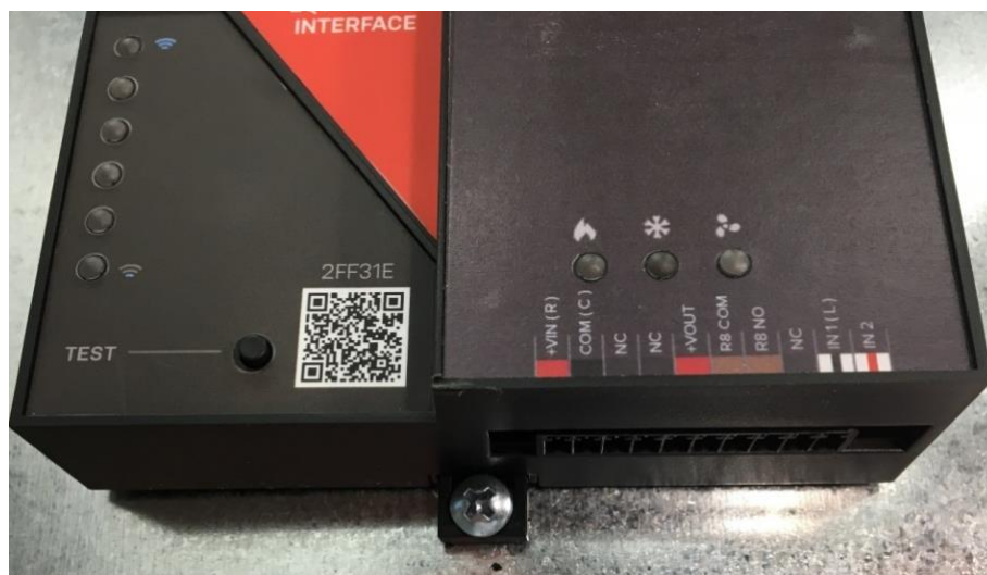
Figure 22: The DIN clip on the bottom is shown secured with the #8 screw:
