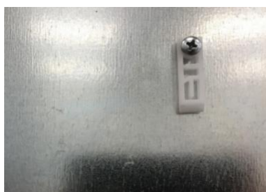
Figure 20: Top DIN Clip is shown mounted first to avoid any metal shavings from dropping in to the case.
