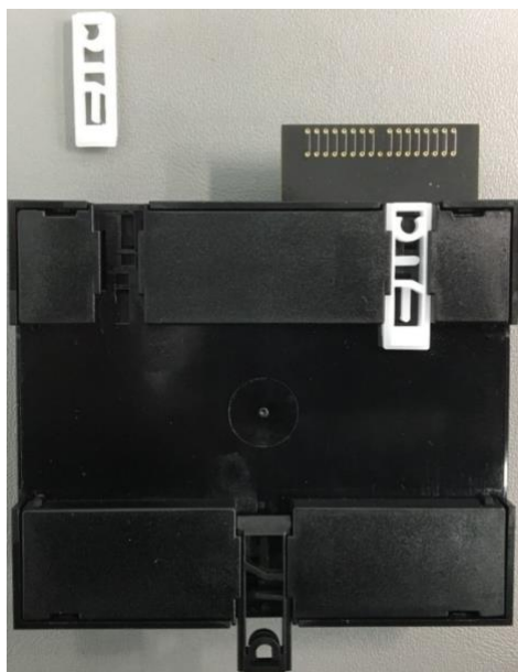
Figure 20: Top DIN Clip is shown mounted first to avoid any metal shavings from dropping in to the case.
